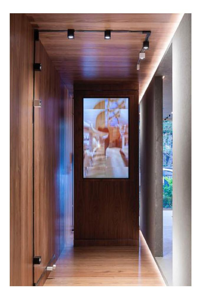
The system is made of an advanced 6 mm thick conductive track that winds through space carrying a 48V current on which light units can be attached Different connectors can be installed on the power track using simple magnets making it possible to combine different modules easily and simply.
