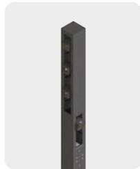
Ideal for wide walkways, access roads, ramps or any other area that requires long and narrow lighting. The optical system has a 25° beam opening, ideal for lighting areas up to 4 times the width of the installation height and 1.75 times the depth. In a single pole configuration, the 350cm pole has a distribution of 14m and a 500cm pole has a distribution of 20m.
