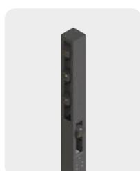
The marked asymmetrical optic has a 60° beam opening, making it the most suitable solution for lighting both horizontal planes like parking areas, as well as vertical surfaces like building facades. It is ideal to light areas up to 2.75 times the installation height. In a single pole configuration, the 350cm pole has a distribution of 9,60m and a 500cm pole has a distribution of 13,75m.
