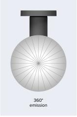
MRS BO Path 150mm produces a single 360° radial emission in four different colour temperatures. It is suitable for step marker lighting.
