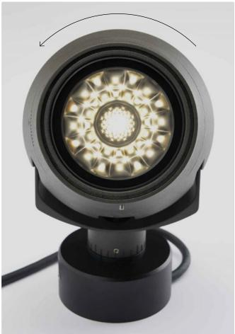
Emission can vary from Spot (20°) to Medium Wide Flood (41°) continuously with mechanical locking of the zoom on the chosen distribution. A practical graduated scale facilitates replication across multiple fixtures.
