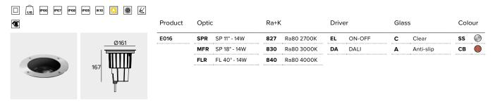
Note All lighting fixtures have to be completed with installation sleeves.
